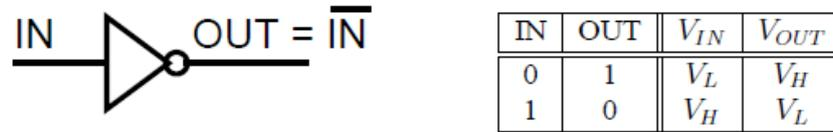
Fig.3. Inverter: symbol and truth table
