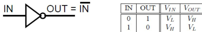
Fig.3. Inverter: symbol and truth table
