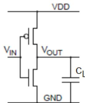
Fig.6. A CMOS inverter with an equivalent load capacitance
