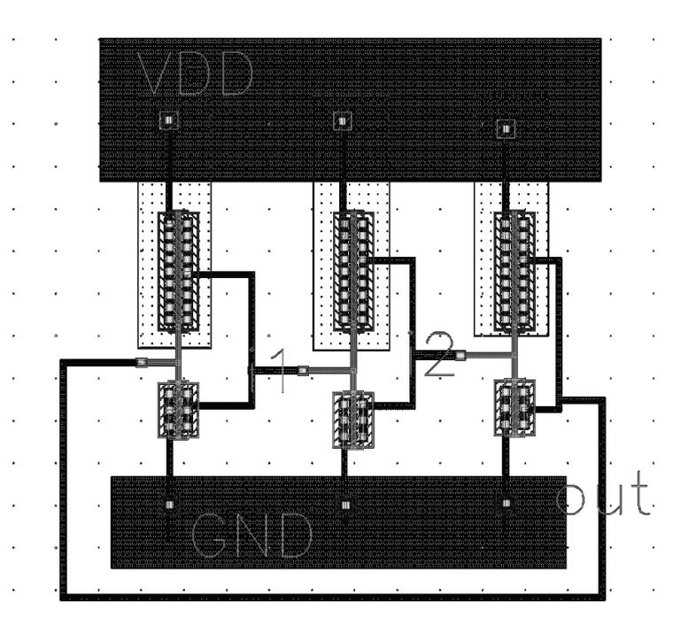
Fig.8. Ring oscillator - layout
