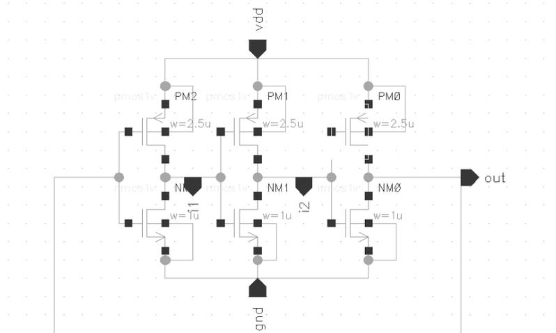
Fig.7. Ring oscillator schematic
