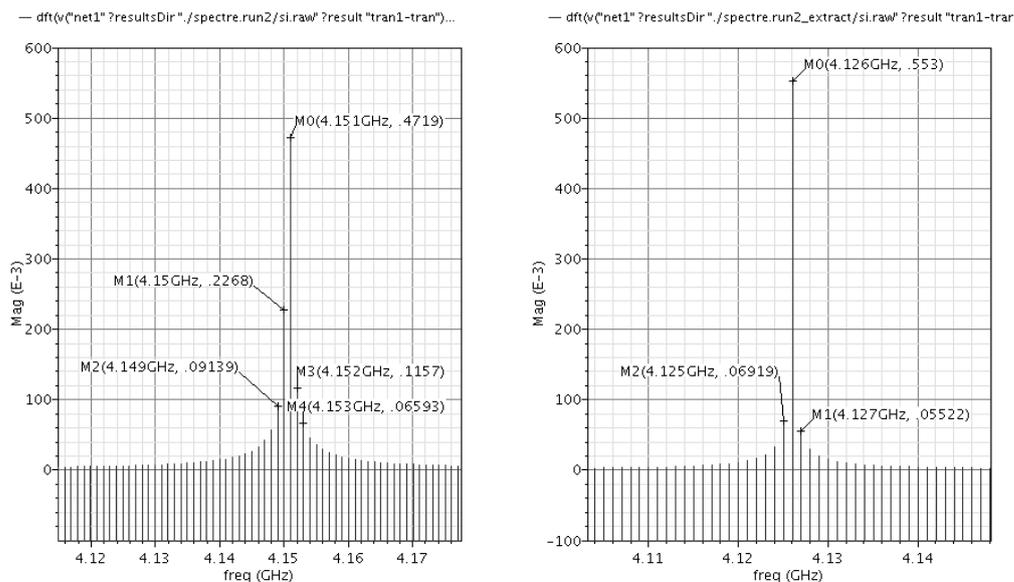
Fig.17. Oscillation frequency without (left) with parasitic parameters (right)
