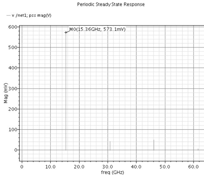
Fig.18. Oscillation frequency for a load capacitance of 10fF
