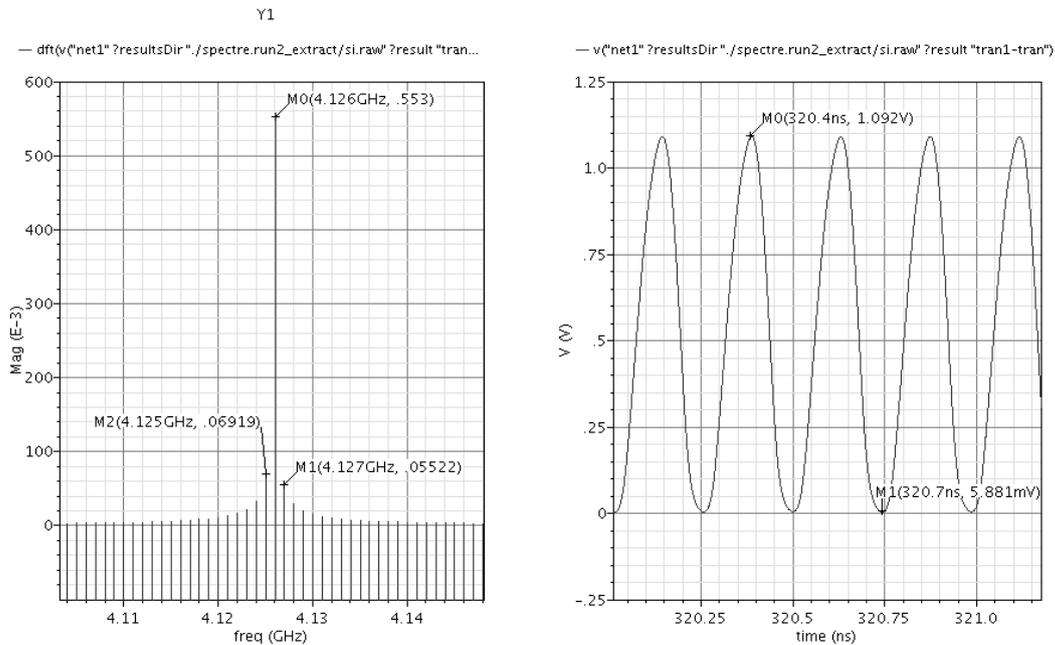
Fig.16. Output voltage in frequency and time domain including parasitic parameters
