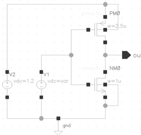
Fig.4. CMOS Inverter circuit in Cadence
