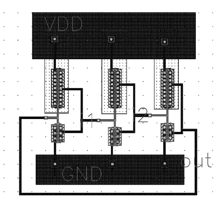
Fig.8. Ring oscillator - layout
