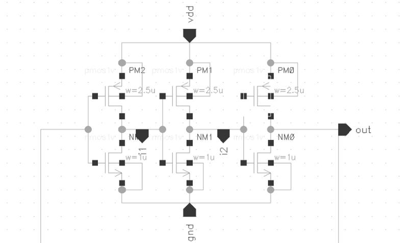
Fig.7. Ring oscillator schematic
