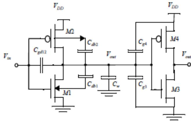
Fig.9. Parasitic Capacitances
