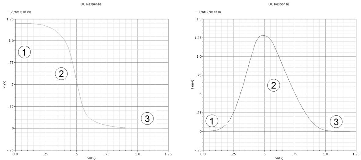
Fig.5. The transfer (left) and current (right) characteristics of a CMOS Inverter
