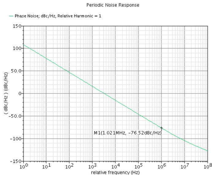
Fig.19. Phase noise by a frequency offset  $f=1$ MHz
