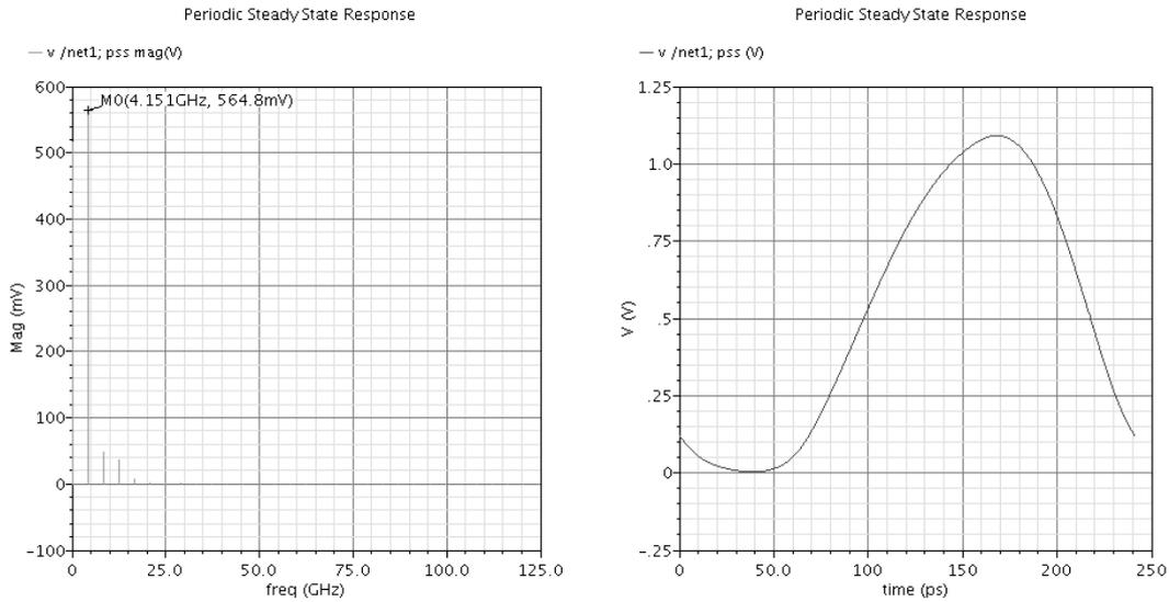
Fig.12. Output voltage in frequency and time domain
