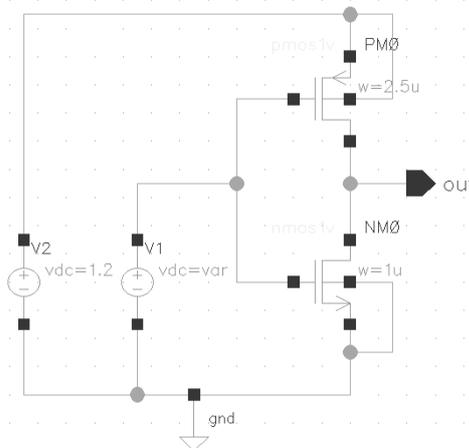
Fig.4. CMOS Inverter circuit in Cadence
